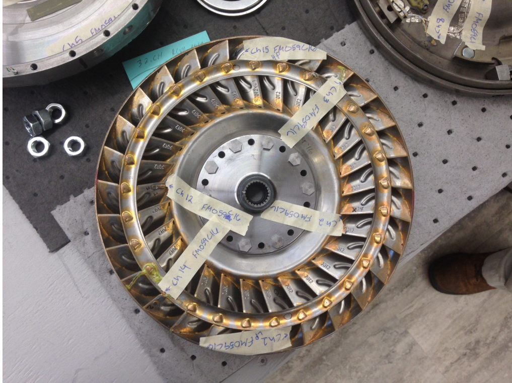
Figure I-31. Turbine transducer locations
