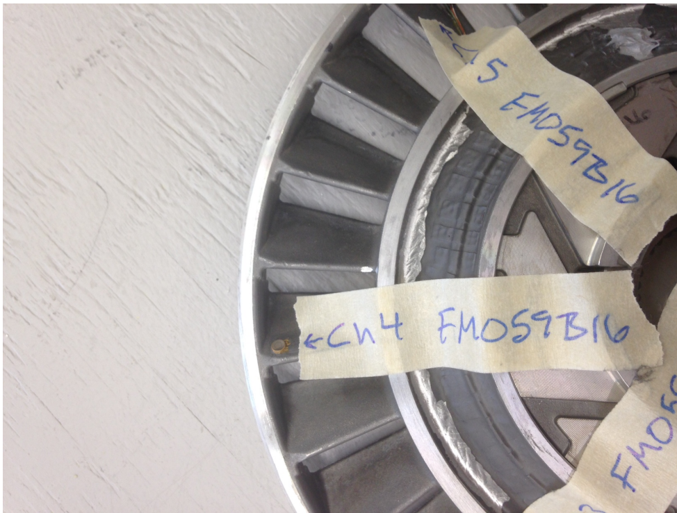
Figure I-26. Stator channel 4 location, leading edge/core/pressure side
