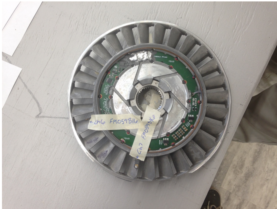
Figure I-28. Stator transducer locations
