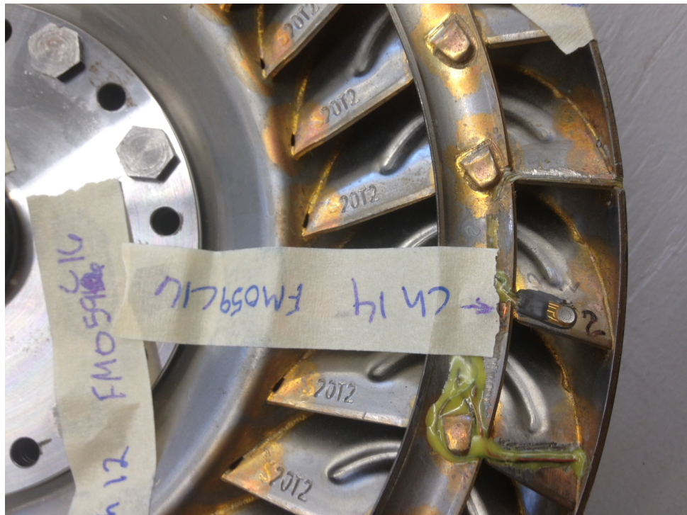
Figure I-36. Turbine channel 14 location, leading edge suction side
