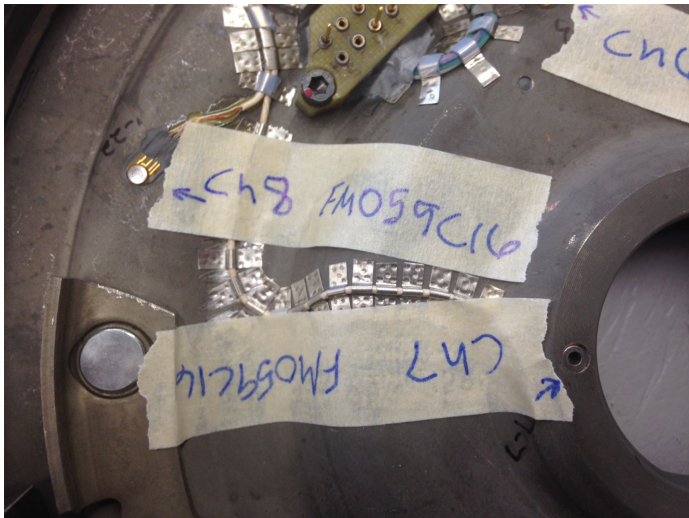
Figure I-46. Clutch channel 7 and 8 locations, inner and outer radius respectively
