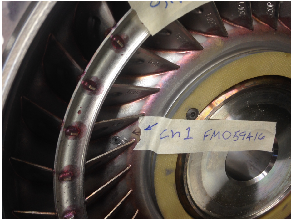
Figure I-16. Impeller channel 1 location, leading edge between blades
