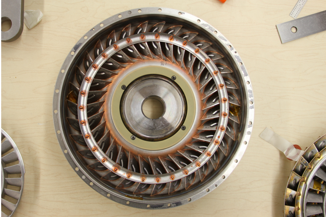
Figure I-11. Impeller with stator transmitter induction coil
