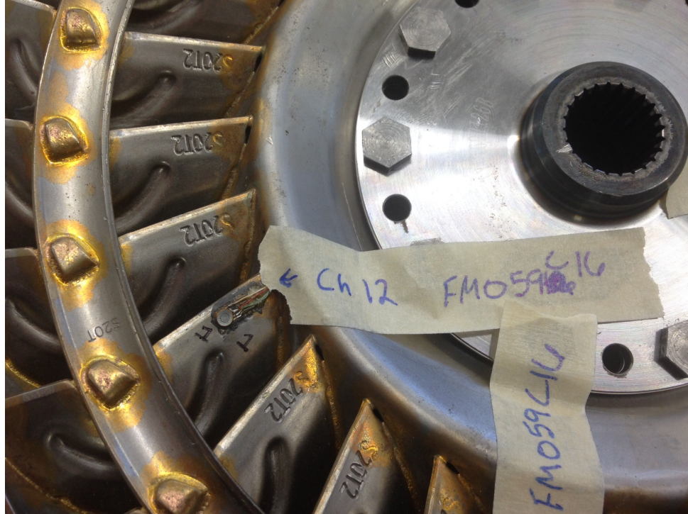
Figure I-35. Turbine channel 12 locations, trailing edge suction side
