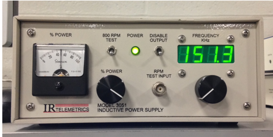
Figure I-1. Power supply for telemetry
