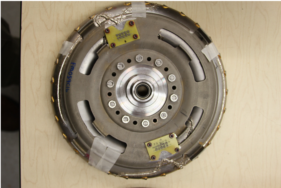
Figure I-6. Power and signal pin arrays mounted to shell of turbine
