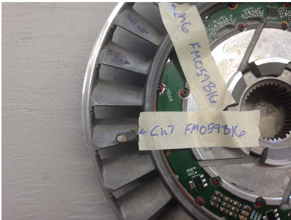
Figure I-30. Stator channel 7 location, trailing edge/middle/suction side
