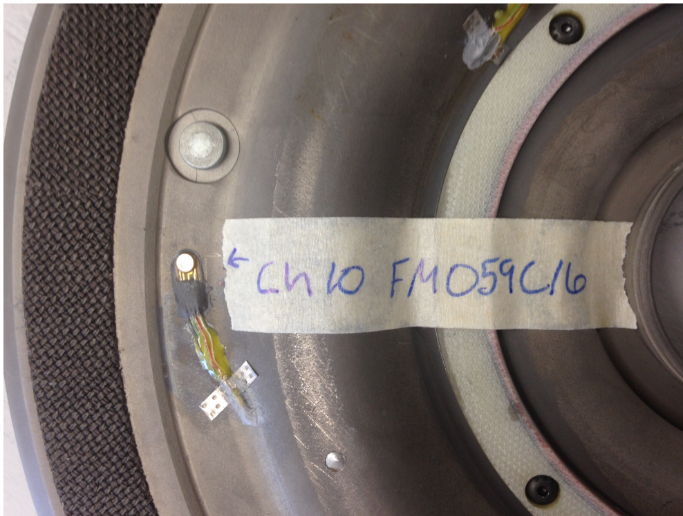
Figure I-42. Clutch channel 10 location, outer radius before friction material
