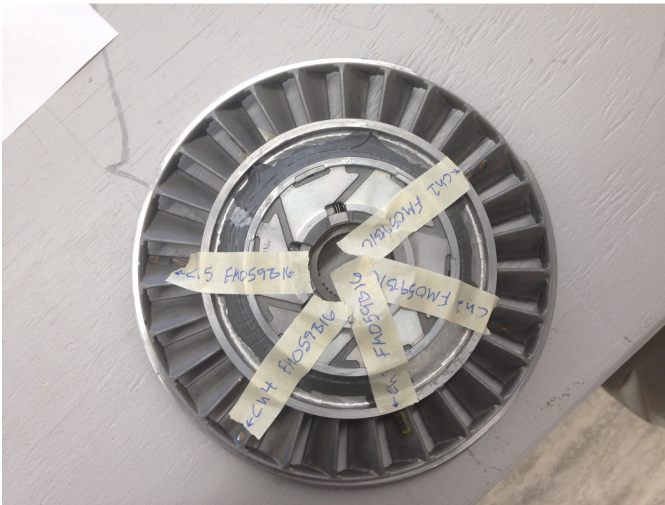
Figure I-22. Stator transducer locations
