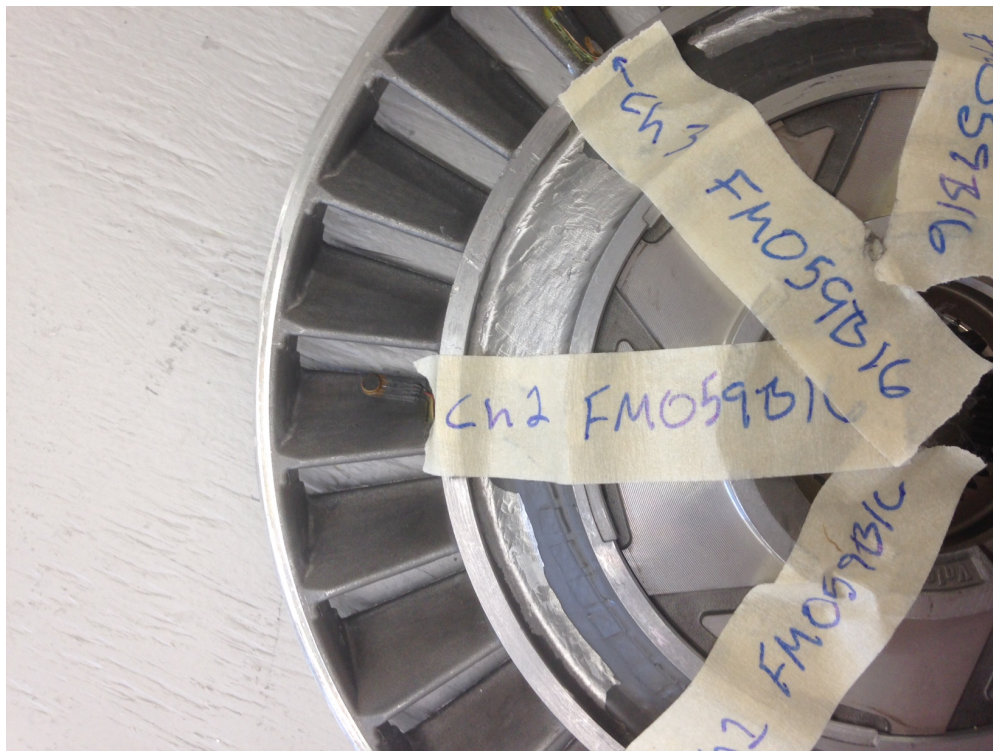
Figure I-24. Stator channel 2 location, trailing edge/middle/pressure side
