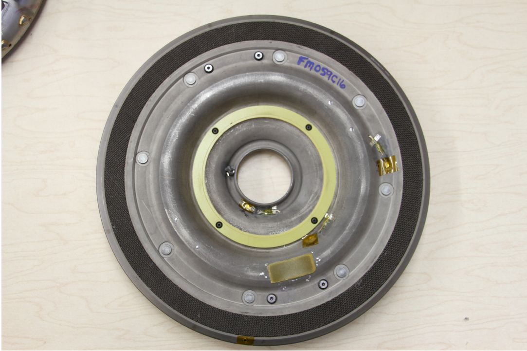
Figure I-5. Kevlar patch on clutch plate for transmitter
