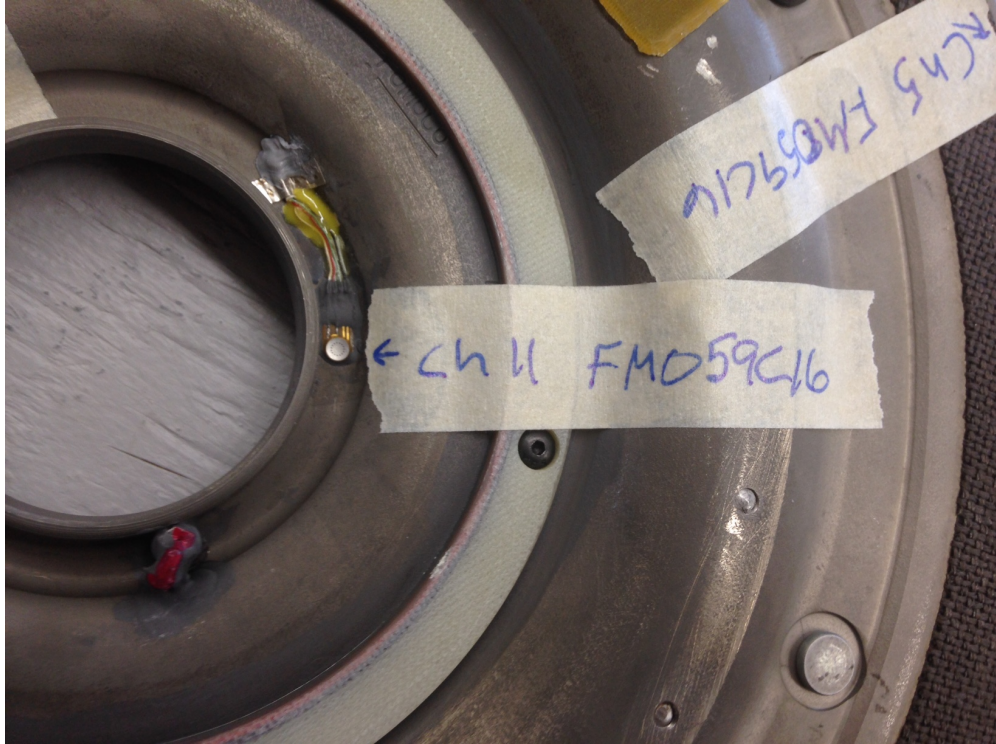
Figure I-43. Clutch channel 11 location, inner radius
