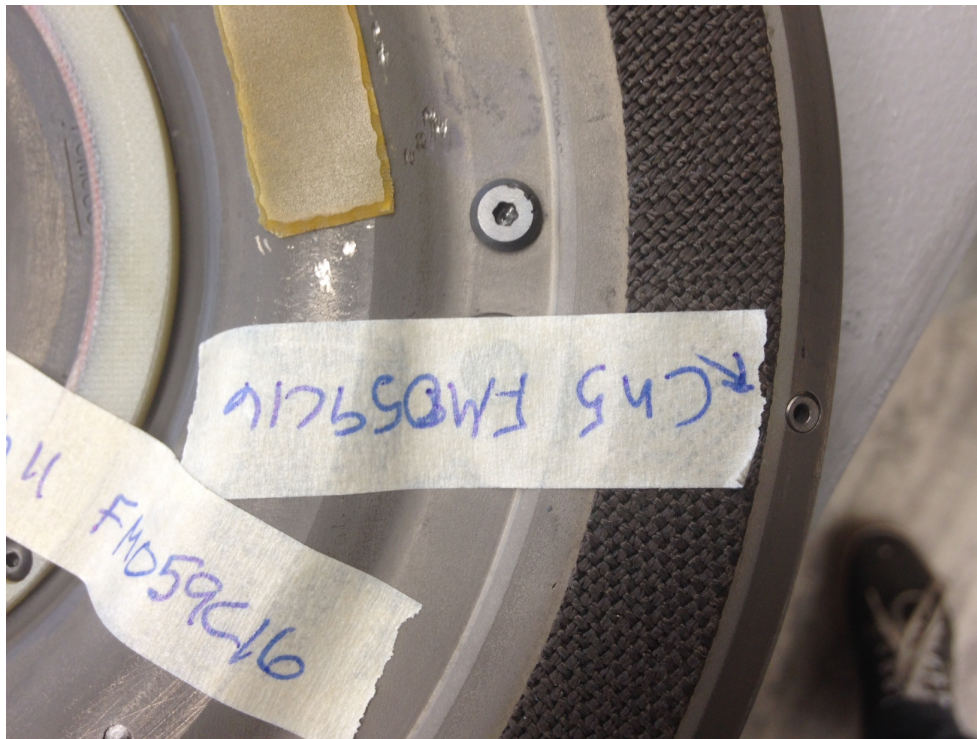
Figure I-40. Clutch channel 5 location, outer radius past friction material
