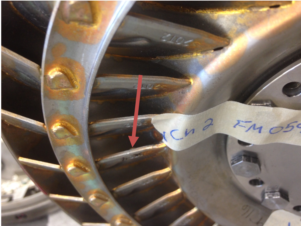
Figure I-33. Turbine channel 2 location, trailing edge pressure side
