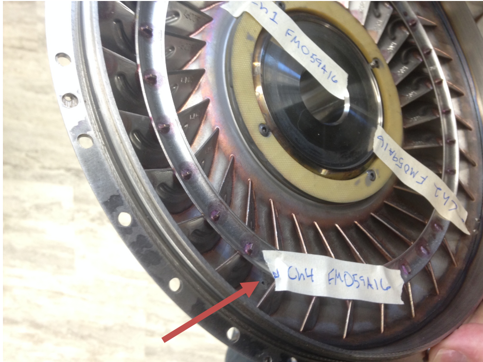
Figure I-19. Impeller channel 4 location, center between blades
