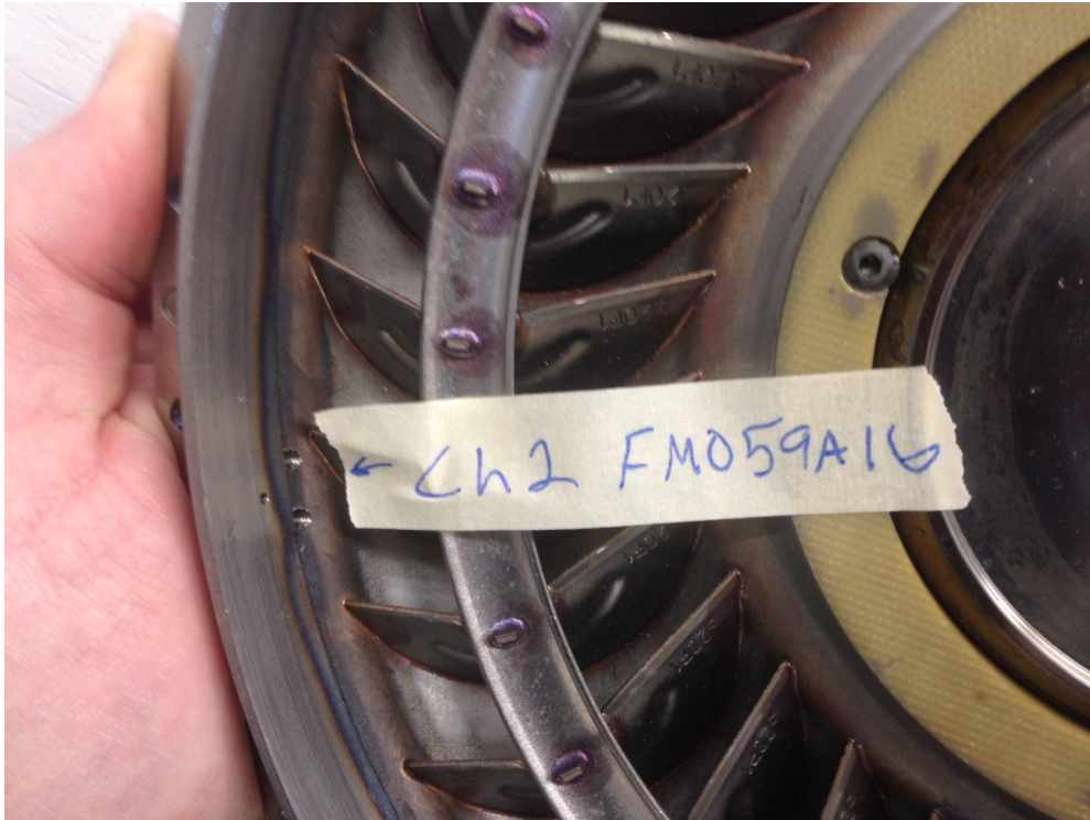
Figure I-17. Impeller channel 2 location, between impeller and turbine
